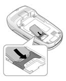
Note: When you need to remove the SIM card, slide it, as shown, and take it out of the socket.
